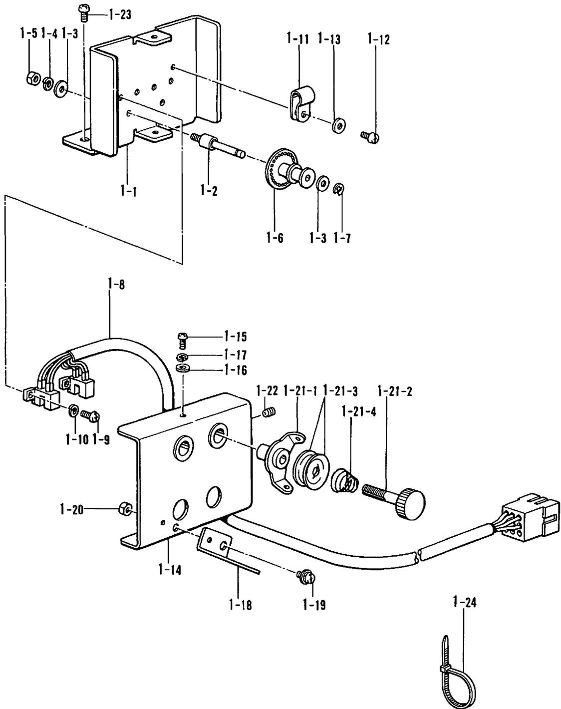
J. 糸切れ感知関係/Thread breakage detector mechanism/Fadenbruchfühler/
