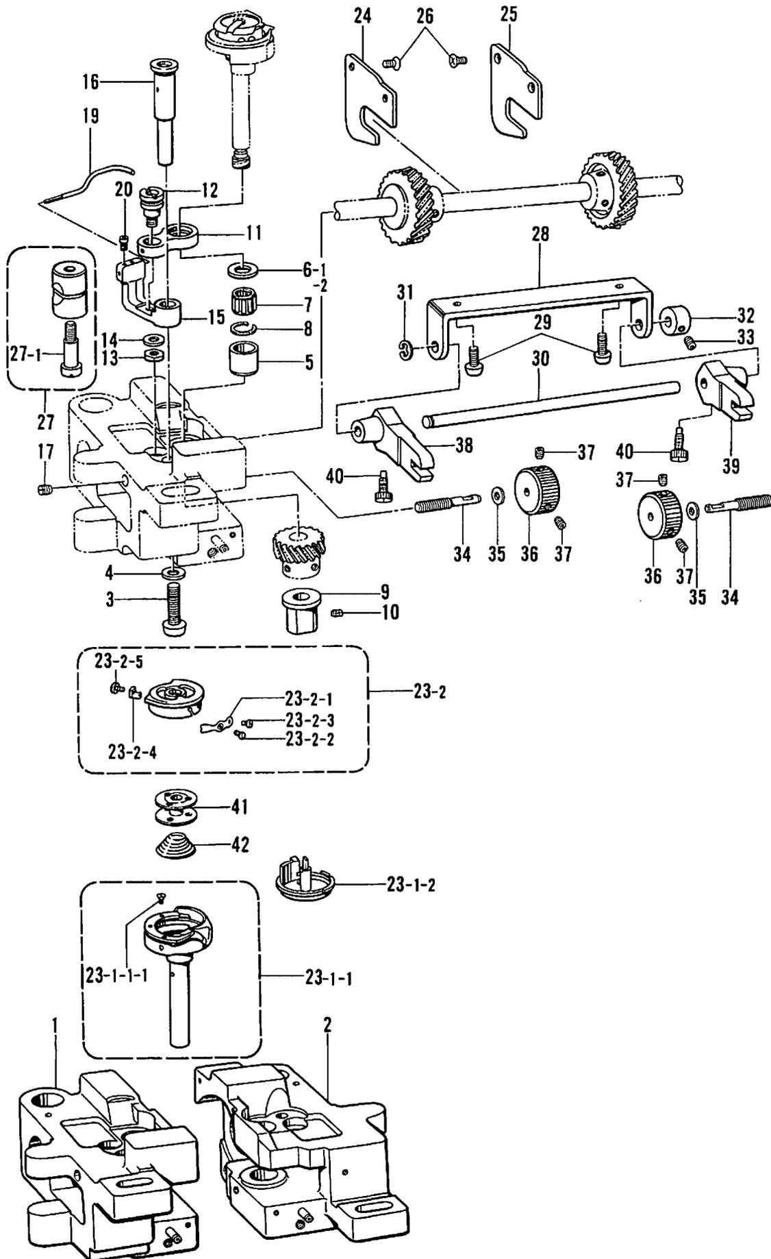
F. カマ関係/Rotary hook mechanism/Greifervorrichtung/
