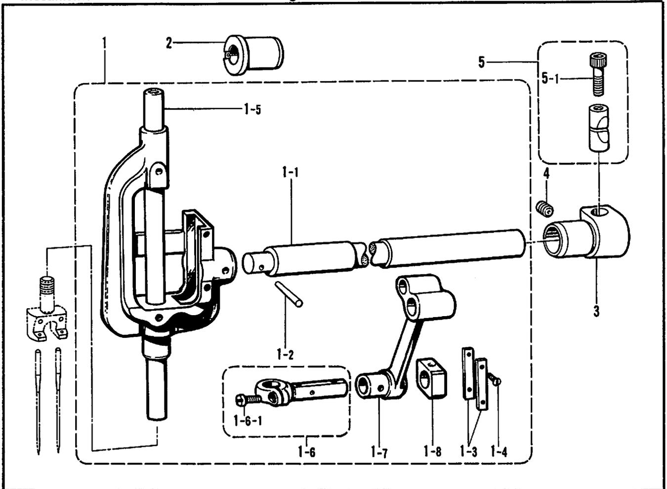
D. 下軸關係/Lower shaft mechanism/Untere welle/
