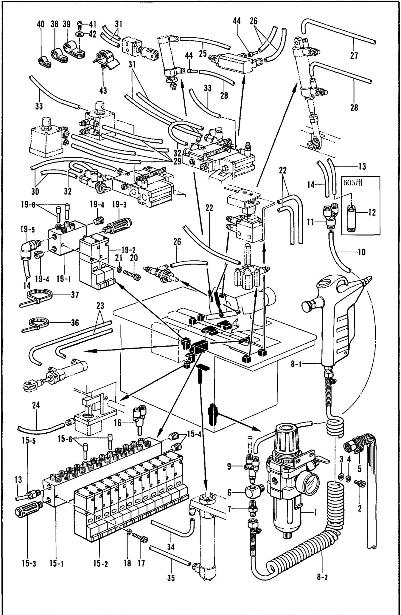
P. 空圧関係/Air pressure mechanism/Luftdruck/
